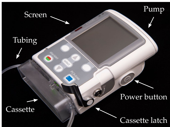
Connecting the tubing to the pump.
