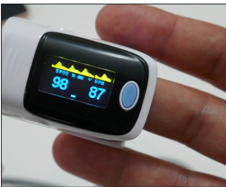
A pulse oximeter shows the amount of oxygen in your blood.
