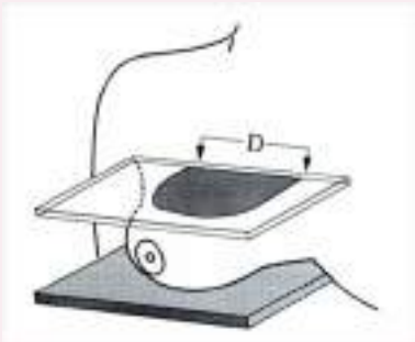
Figure 8-11 Compression in pounds per square inch (psi). The actual pressure applied to the breast is the force applied (in pounds) divided by the area over which the force is spread, giving psi. If the breast is assumed to be a hemisphere, then psi equals half the area of a circle whose diameter (D) is that of the part of the breast touched by the compression paddle, divided into the number of pounds applied. This diagram depicts the surface in contact with the compression paddle and film holder. The larger the surface in contact, the lower the pressure in psi.
